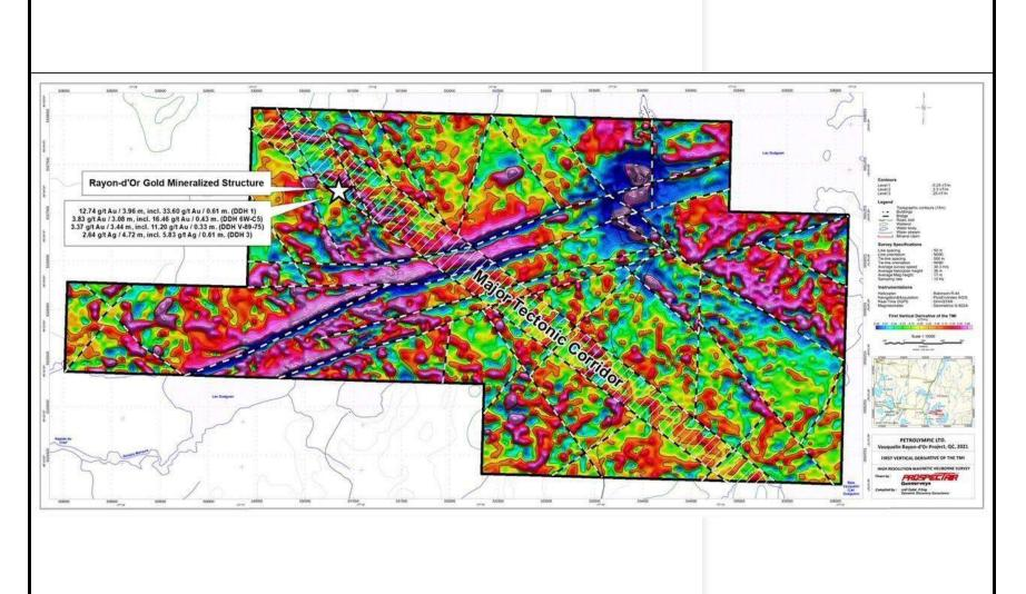
High resolution heliborne magnetic survey undertaken by Petrolympic in 2022, revealing potential favourable host structures for mineralizations.
