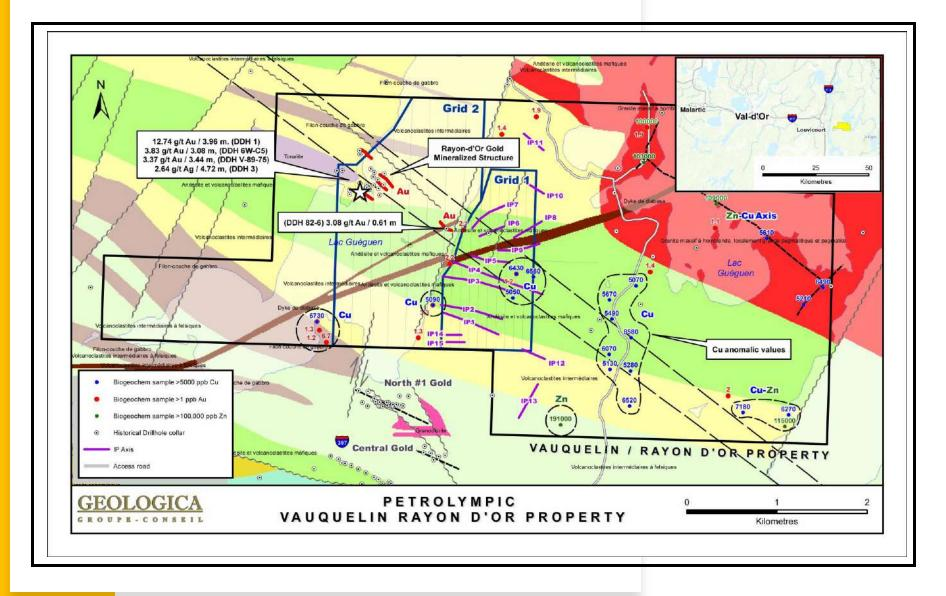
IP and magnetic surveys indicate the presence of numerous structures and the extension from Rayon d'Or into Vauquelin, coinciding with gold, copper and zinc biogeochemical anomalous values.
