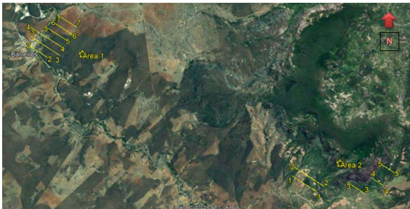
Figure 9-6 Location of the Lines and Measuring Stations of the Chargeability and Resistivity data of Area 1 and Area 2 of the Lithium Project
